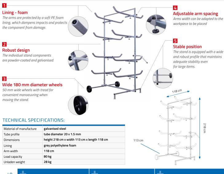
**VERSATILE USE** SOFT PROTECTIVE LINING ADJUSTABLE ARM SPACING
