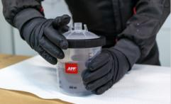
Place the cap on the hard cup and tighten it until it stops.
