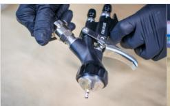
Attach the appropriate FPS connector on a spray gun to the cup connector. The connection must be tight and mechanically resistant.
