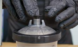
Disconnect the cup from the gun, performing assembly steps in reverse. Close the spout of the soft cup tightly with the cap. Unscrew the cap from the hard cup and remove the soft cup with the cap. If you have trouble removing it, push it gently upwards through the hole in the bottom of the hard outer cup.
