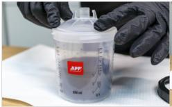
Place the lid with integrated filter on the soft cup and press it down as far as it can go. The connection to the soft cup must be tight.
