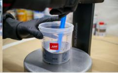
Mix the paint according to the recipe and mixing ratio for the ready-to-spray paint mixture.
