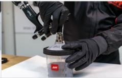
Place the FPS connector previously fitted to the gun onto the spout of the standing cup and press it down as far as it goes; then rotate it by ¼ turn.
