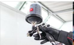
When painting, it is possible to work at any spray gun angle up to and including 180°.
