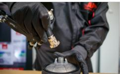
After spraying, disconnect the compressed air hose, turn the spray gun upside down and depress the trigger of the spray gun so that the paint flows out of the gun and back into the cup.
