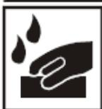
Surfaces covered with factory-made lacquer coats and primers - polish wet using P360-P400 abrasive paper.
