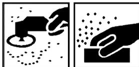
Thoroughly remove corrosion spots.
