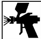
Apply with a spray gun equipped with a  $\varnothing 1.2$ - $\varnothing 1.4$  mm nozzle at an air pressure of 2.0 to 3.0 bar.
