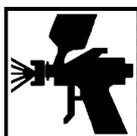
Apply with a spray gun equipped with a  $\varnothing 1.3$ - $\varnothing 1.5$  mm nozzle at an air pressure of 2.0 to 3.0 bar.
