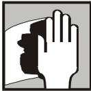
Remove any corrosion centers from raw sheet metal bodywork. Sanding of large, smooth surfaces significantly improves adhesion of the compound to the substrate. It can be applied on bare metal, but for additional protection it is recommended to use anti-corrosion primer. Before spraying, sand the surface to be protected, remove any dust, and, if possible, degrease it using APP W900 remover.
