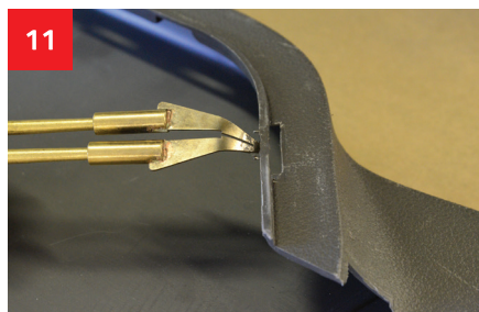
11 Hiding the protruding ends of the staples using the hot tip, as much as possible.
