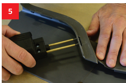
5 Embedding the staple into the damaged area.
