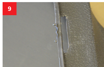
9 The staples' ends still protruding after cutting should be ground (e.g. using a grinder APP No. 139102).
