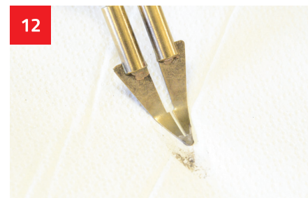
12 Cleaning the tip, if necessary.
