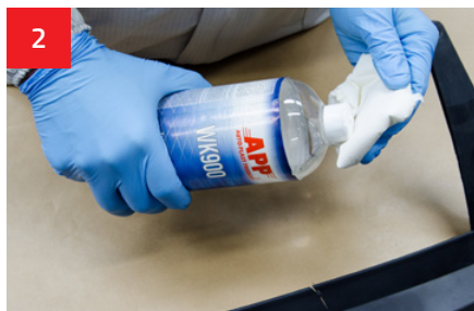
2 Clean and degrease the surface with WK900 Stripper.
