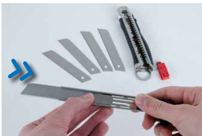
4 - Place blade in storage and insert it into the body
